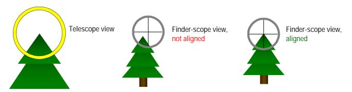
The finder-scope is now aligned to the main telescope. You can check and refine alignment on a night sky object like a star if required. Please note that the view will not be the right way up and views will differ depending whether a diagonal is used or not. If you do not use a diagonal you may need an extension tube to reach focus.
