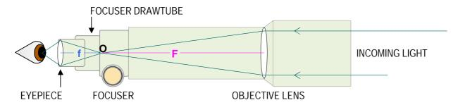
Magnification depends on two factors. The focal length of the telescope and the focal length of the eyepiece used. To calculate the magnifying power an eyepiece gives, simply divide the focal length of the eyepiece into the focal length of the telescope.
